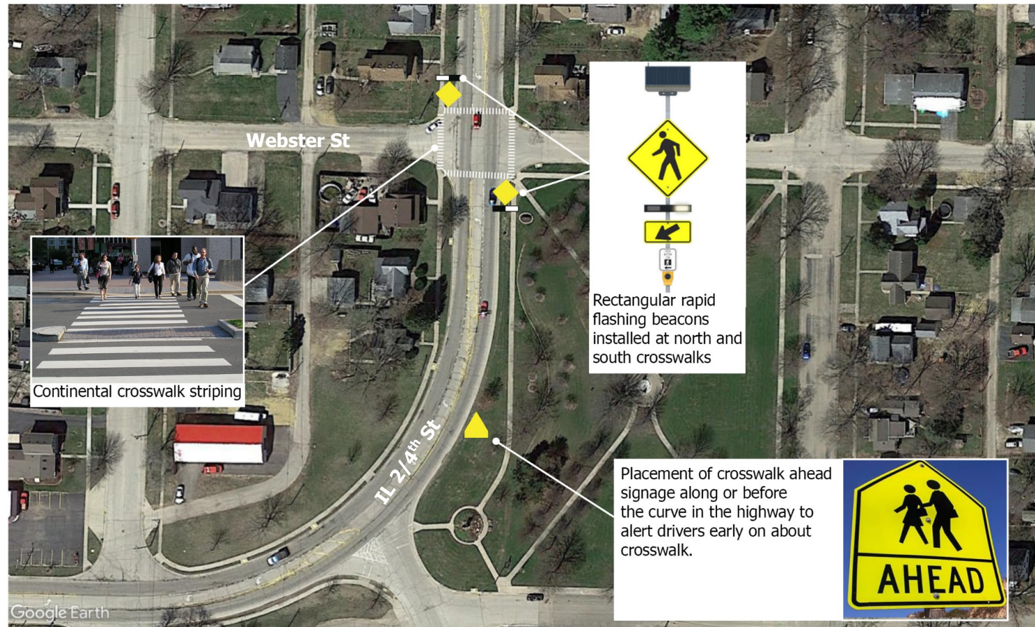
Diagram showing potential improvement options at IL 2/4 th St and Webster St
